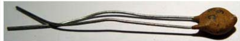
Condensator C1: 5pF
