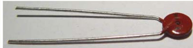
Condensator C2 : 100pF
